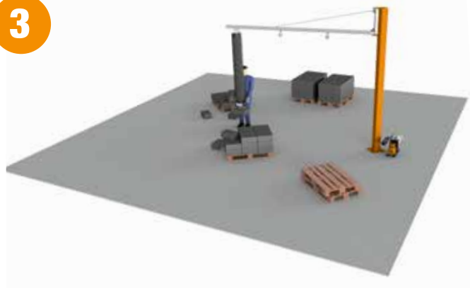
Pillar-mounted slewing jib crane with trolley for floor installation
